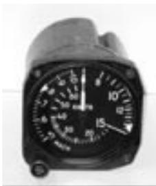
*Typical mechanical airspeed in an early Learjet manufactured by Bendix Aviation Corp.*
