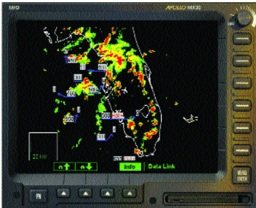
**WSI's NEXRAD** product on UPSAT's MX20 Bezel uses a broadcast satellite system to transmit every product they offer in about two minutes.
