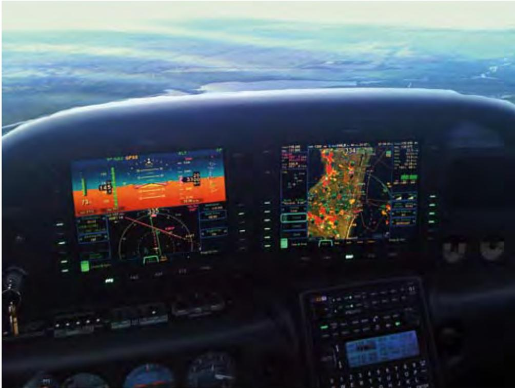
*A customer-owned Cirrus SR22 flies with the first installation of Avidyne's new Entegra Release 9 integrated display system, complete with the new control unit and the advanced PS Engineering audio-control panel, which also integrates with the R9 package.*
