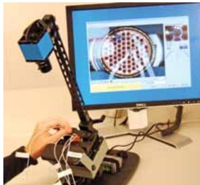
*An operator inserts wires into a connector using Pin-Sight*
