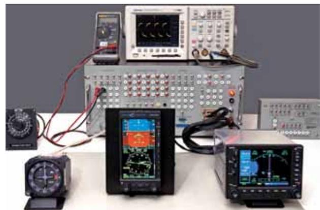
San Luis Avionics' Integrated Avionics Test Panel
