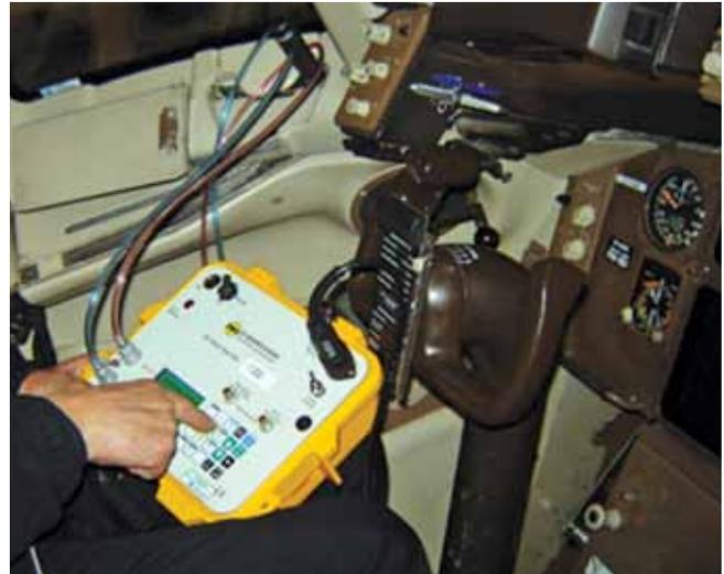
*DMA-Aero's MPS43 Ultra Compact Air Data Test Set weighs 9 pounds.*
