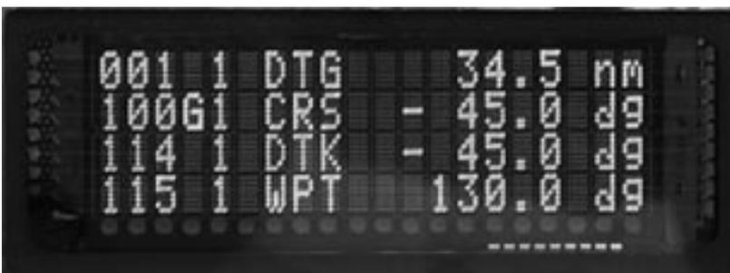
*Label 001, Distance to Go (DTG); Label 100G, Selected Course (CRS); Label 114, Desired Track (DTK); Label 115, Waypoint Bearing (WPT)*
