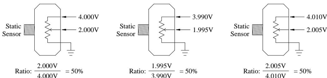
**Figure 1** Ratiometric ratio stays the same if voltage supply varies.
