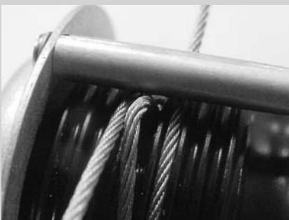
Results of loose primary and bridle cable.
