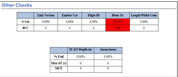
\*In dual band installations (GDL 88 UAT plus GTX w/ES transponder), failure may be only 50%.
