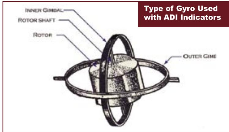
is used in the ADI to establish a reference point to measure change in the attitude of the aircraft around the aircraft's longitudinal (roll) axis and the lateral (pitch) axis of the aircraft. Any movement of the aircraft around the pitch or roll axis of the aircraft will be transferred mechanically or electronically to a miniature airplane and an artificial horizon on the face of the ADI indicator, mimicking the actual relation of the aircraft to the true horizon.
