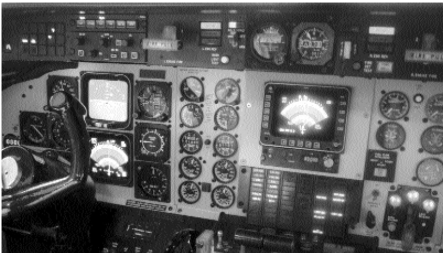
EFIS Flight Deck with RADAR test pattern on EHSI and MFD
