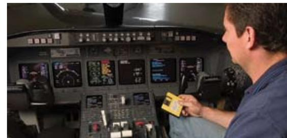
*A Landmark Aviation technician downloads engine and systems data onto a disk for troubleshooting.*
