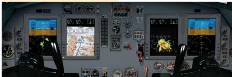
*Rockwell Collins four-display Pro Line 21 installed on a Falcon 20.*
