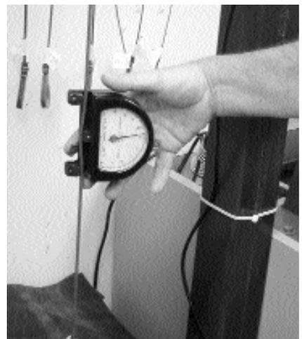
*Calibrating a cable tensiometer*
