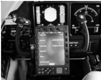
CMC Electronics CT-1000 mounted in a Gulfstream
