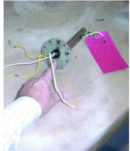
*Defective potted feed-through on stand-off assembly.*
