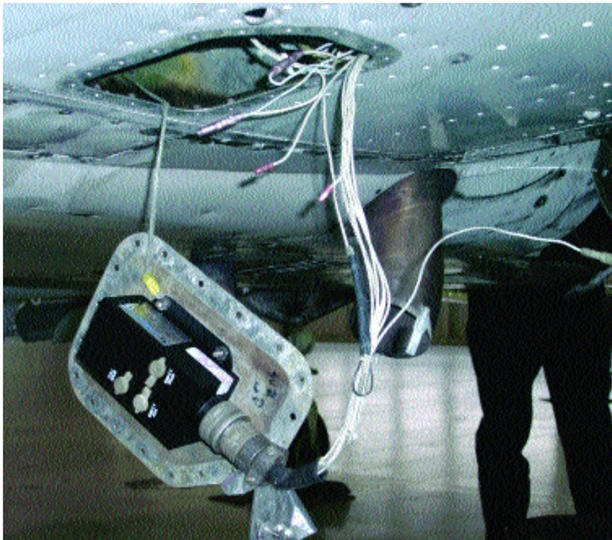
*Signal Conditioner, note the adjustments marked on case.*
