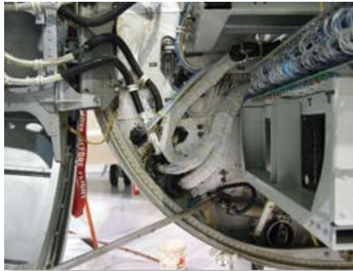
*Premier Air Center/ West Star Aviation gives this Falcon 50 the four-tube EFI-890R installation, including Vision-I, Class A TAWS, dual UNS-1E FMS, P-880 radar, Collins AH-3000 AHRS, dual Universal radio control units, and dual Baker M-1035 audio panels.*
