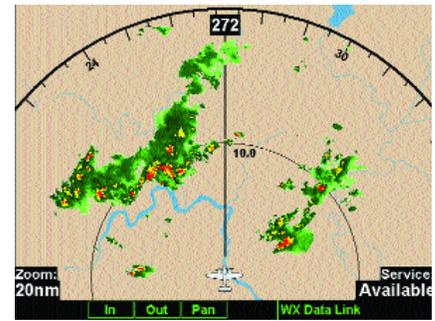
*NEXRAD graphic as seen via the Capstone Universal Access Transceiver (UAT) data link system.*
