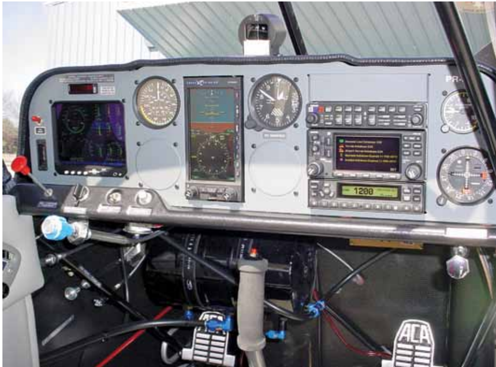
When cross-country capabilities are more important than weight, American Champion combined a JPI 930 engine monitor, Aspen EFD1000, with Garmin 347 audio panel, GNS430W and GTX327 transponder.
