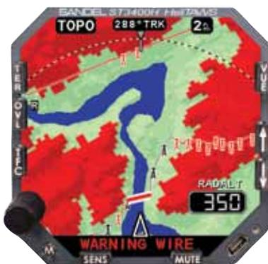
WireWatch has been added to Sandel's ST3400H HeliTAWS terrain avoidance system.
