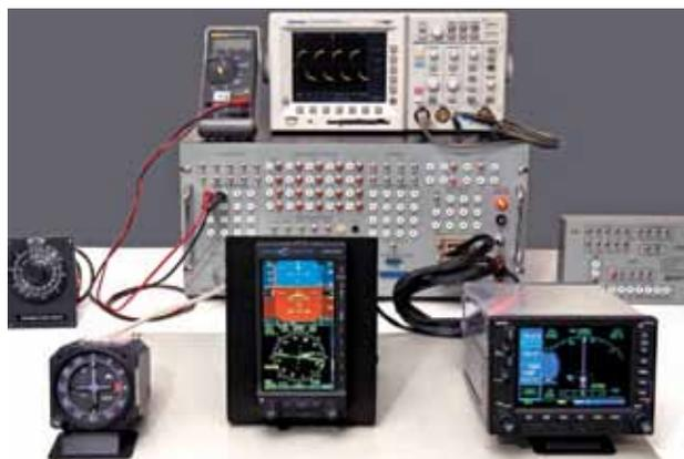
San Luis Avionics' Integrated Avionics Test Panel
