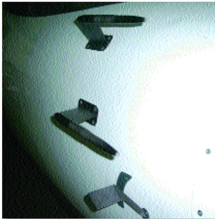
Both pitot tubes contain two static ports. Another pitot tube with dual static ports is on the pilot's side as well.
