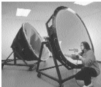
In fact, today's radar systems are so sensitive to changes in their radome's performance that as little as 12 to 15 mils total thickness of additional filler material or paint will reduce the signal efficiency of the system. It's so important that FAA Advisory Circular 43-14 specifically states; "all repairs to a radome, no matter how minor, must return the radome to its original or properly altered condition, both electrically and structurally."
