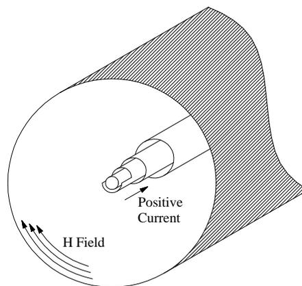
Figure 1 Coaxial cable cut-away showing skin effect.
