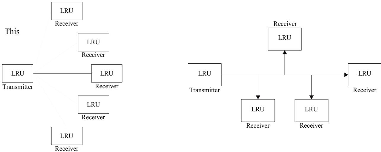
**Figure 1: Star Topology for LRU Wiring (left) and Bus Drop Topology for LRU Wiring (right)**
