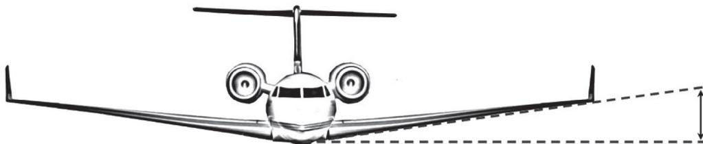
Figure 3. Dihedral is the upward slant of the wings.
