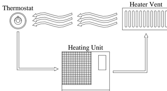
**Figure 1** Furnace shown as example of feedback loop.
